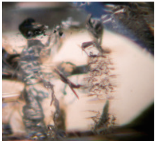
Fig. 3 Dark wormhole-like laser channels seen in fractures extending from the diamond’s surface to the point where an inclusion has been dissolved. This pattern is characteristic of the “KM” treatment. (Photo: Eric Erel)
